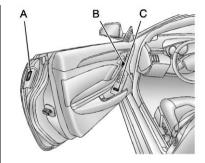
When you have the transmitter with you, you may also unlock and open the door by squeezing the door handle sensor (A). You do not have to press the unlock button on the transmitter. You will be able to open the door when you press the door handle sensor and the vehicle recognizes your keyless access transmitter. When the passenger door is opened first, the driver's door will also unlock.
